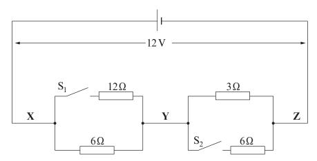
(i) Calculate the resistance of the circuit when both S<sub>1</sub> and S<sub>2</sub> are closed. [3]
